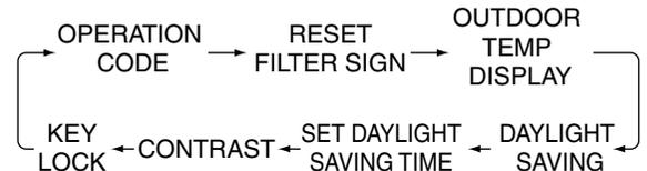
3. In the Outdoor Temp Display setting screen, press the  $\triangleleft$  or  $\triangleright$  button (3) to display or hide the temperature indication.
