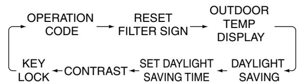
3. In the Reset Filter Sign screen, select the air conditioner for which the filter sign is to be reset by using one of the individual group selection buttons (3).
