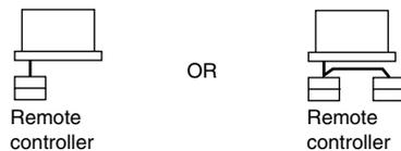
3. Up to 16 indoor units group-controlled by one or two remote controllers
