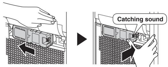
② Make sure the hook is facing to the right, and insert the connector as deeply as it will go.
