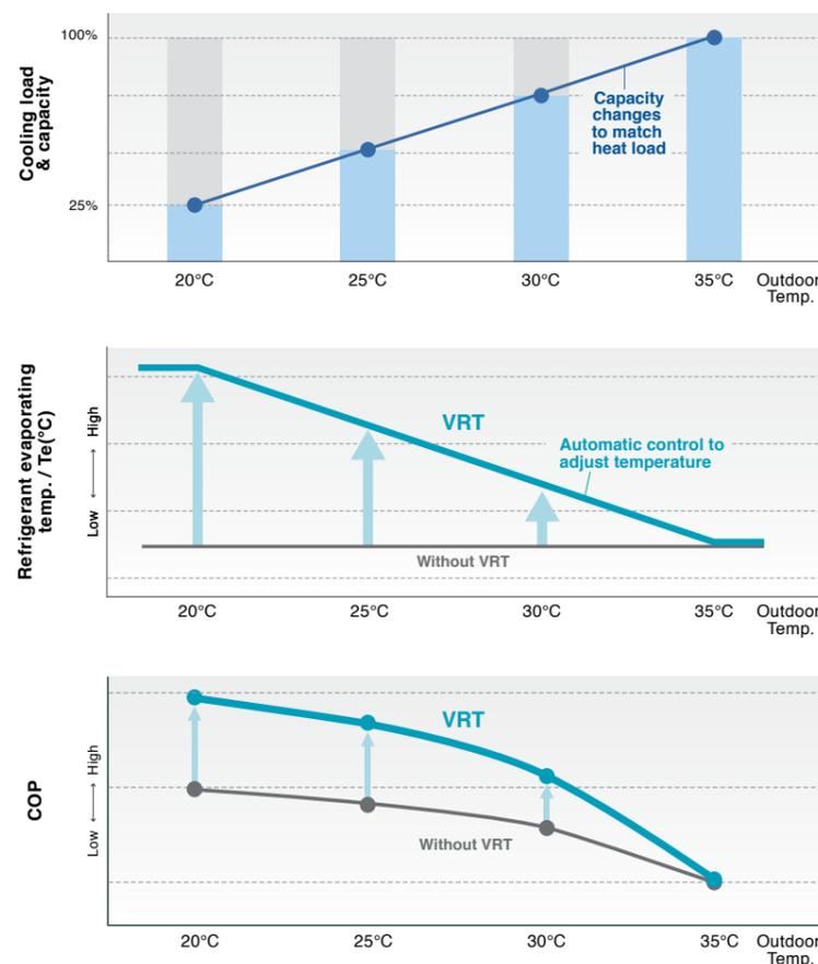
Required capacity changes as air conditioning load changes according to outdoor temperature.
