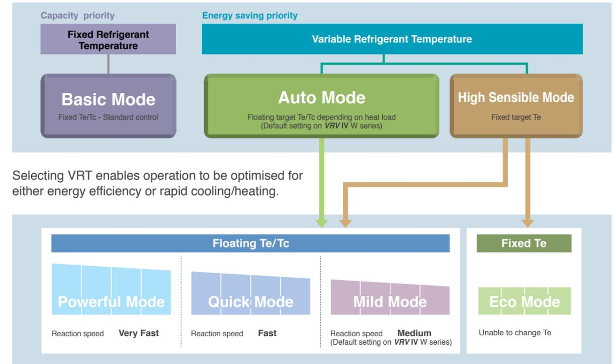
Selecting VRT enables operation to be optimised for either energy efficiency or rapid cooling/heating.
