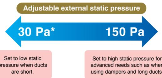
Comfortable airflow is achieved in accordance with conditions such as duct length.
