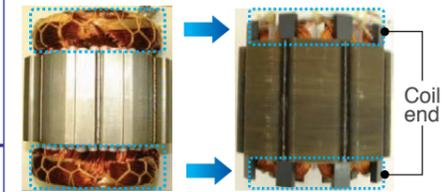
Small sizing coil end using concentrated winding, reduce copper loss (winding resistance).
