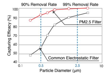
\*Test results by the Heating, Ventilation and Air Conditioning Lab at Tongji University
