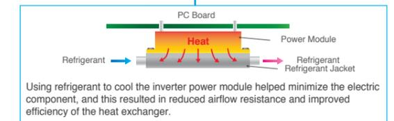
Using refrigerant to cool the inverter power module helped minimize the electric component, and this resulted in reduced airflow resistance and improved efficiency of the heat exchanger.
