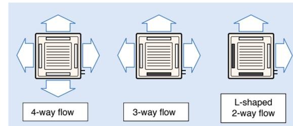
\*For 3-way or 2-way flow installation, the sealing material for air discharge outlet (option) must be used to close each unused outlet.
