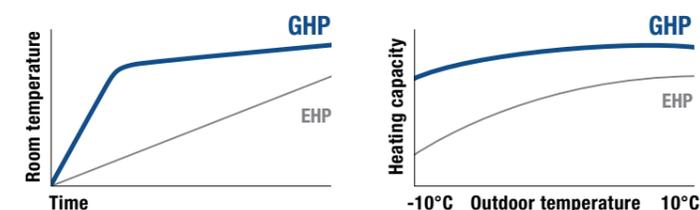
The ability to harness the waste heat from the coolant circuit enables rapid and powerful heating performance. This feature also results in less frequent defrost operation for GHP systems.
