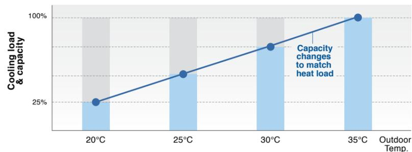
Required capacity changes as air conditioning load changes according to outdoor temperature.
