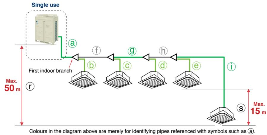
Colours in the diagram above are merely for identifying pipes referenced with symbols such as (a).
