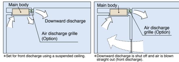
\*Set for front discharge using a suspended ceiling. \*Downward discharge is shut off and air is blown straight out (front discharge).
