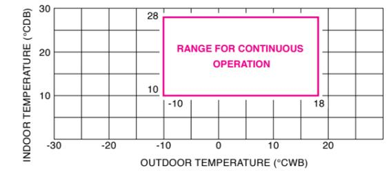
\* If the unit is used out of the operation temperature range (especially at high outdoor temperature), it may malfunction, or the protection circuit may trip and deactivate the unit.
