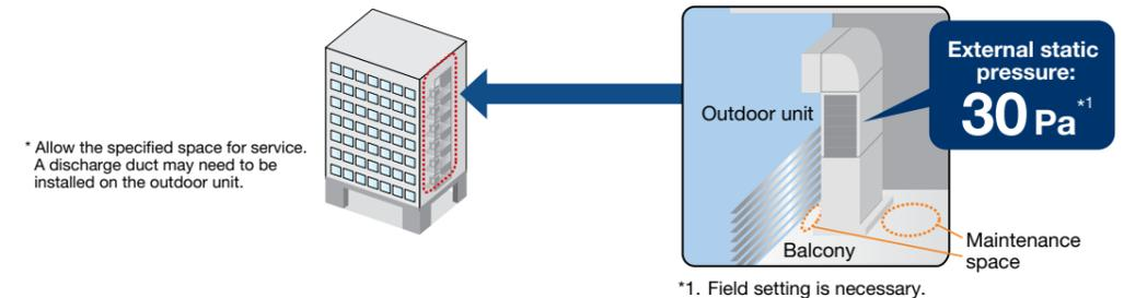
\* Allow the specified space for service. A discharge duct may need to be installed on the outdoor unit.
