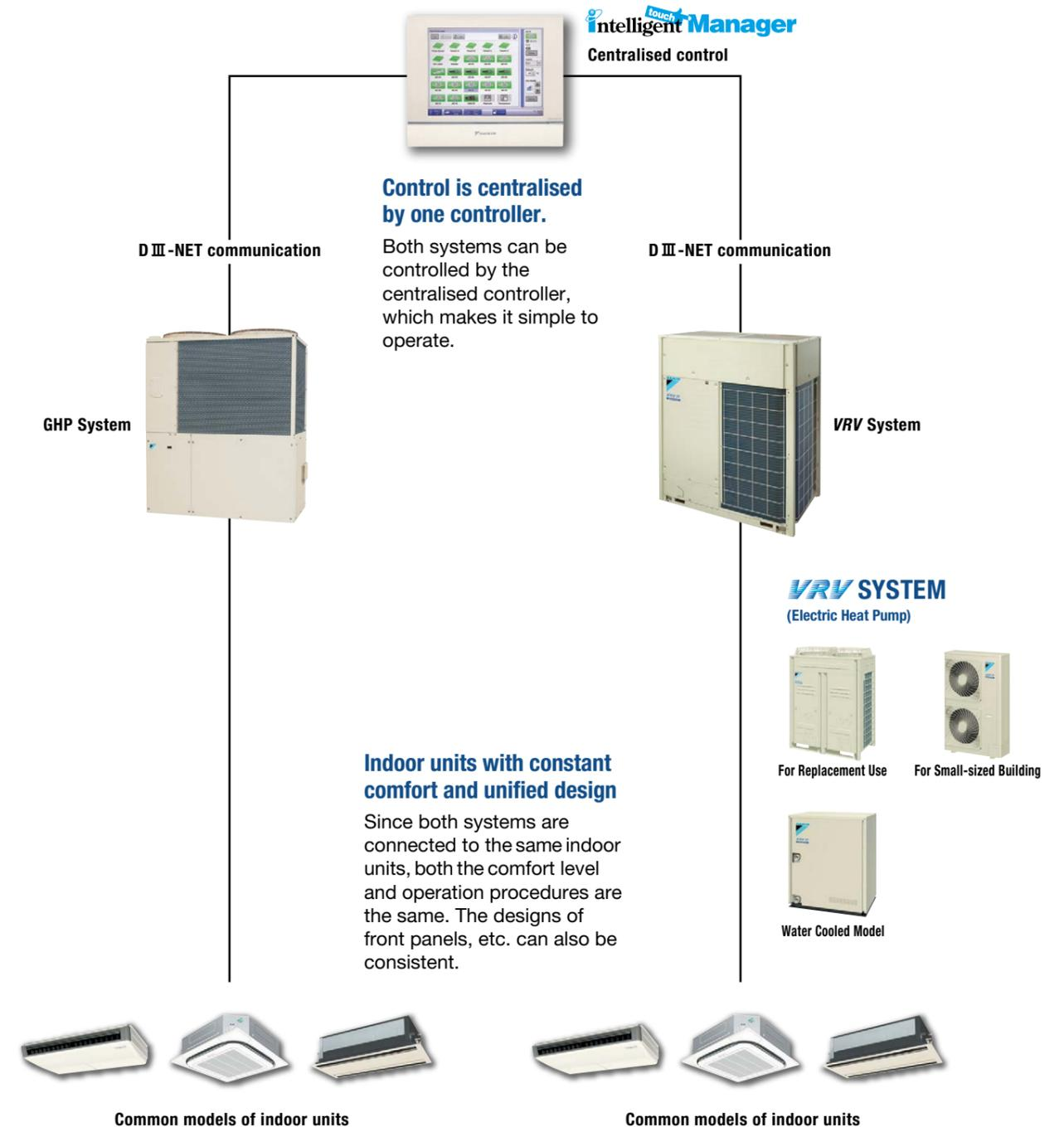
Common indoor models for both GHP and EHP systems ensure a consistent look for exposed units whilst maintaining similar comfort levels and keeping operational control.
