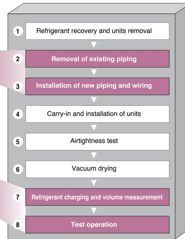
\* For reuse of existing refrigerant piping, it is possible to use piping or branched piping capable of handling 3.3 MPa or more. Thermal insulation is necessary for liquid piping and gas piping.
