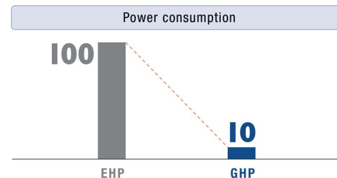
In GHP system, only the condenser fans and the indoor units consume electricity. In comparison to EHP, the electrical power required to operate GHP is significantly less, thereby enabling the electrical substation and switch gear equipment to be downsized compared to EHP.
