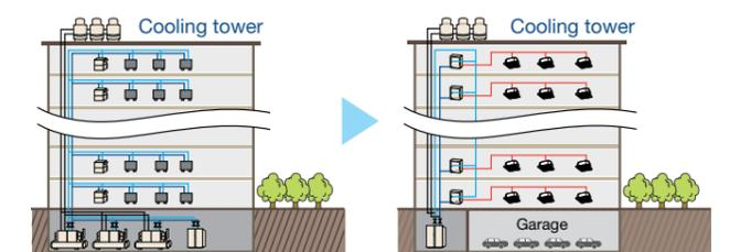
With a conventional central air conditioning system, the outside units take up a disproportionately large amount of space for installation.
