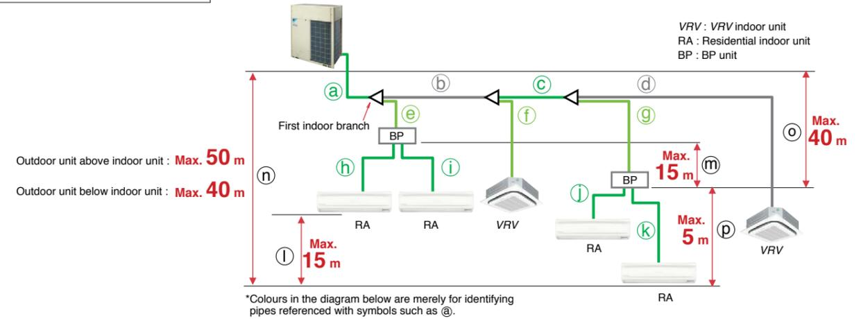
When a mixed combination of VRV and residential indoor units is connected or when only residential indoor units are connected
