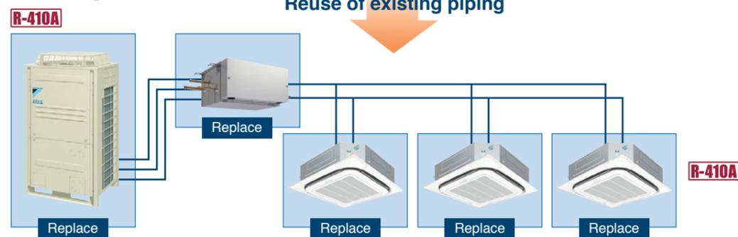
\* It is not possible to combine old R-22 and new R-410A indoor units in one system due to incompatibility of communication. It is not possible to keep R-407C indoor units.
