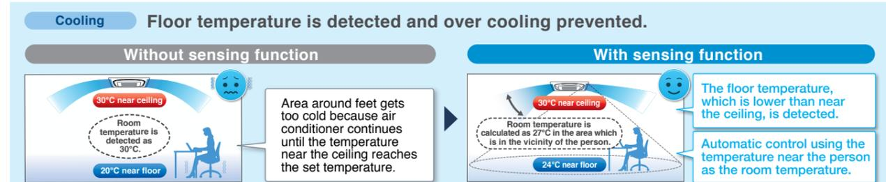
**Energy savings** The temperature near the person is automatically calculated by detecting the temperature of the floor. Energy is saved, because the area around the feet does not get too cold.
