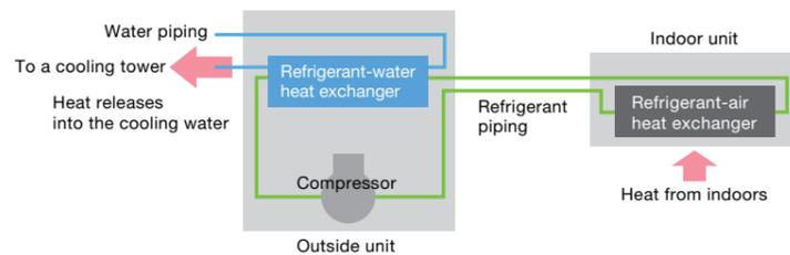
As a water cooled system does not require to exchange heat with outdoor air,
