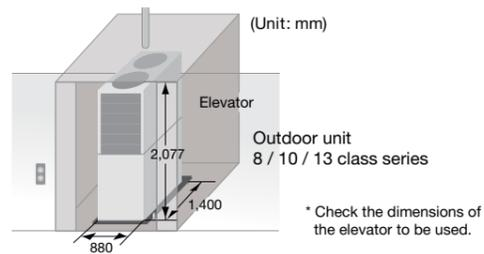
The compact outdoor unit can be installed on the service balcony of each floor.
