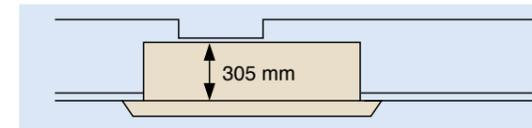
(When a high-efficiency filter is attached, the unit's height is 400 mm.)
