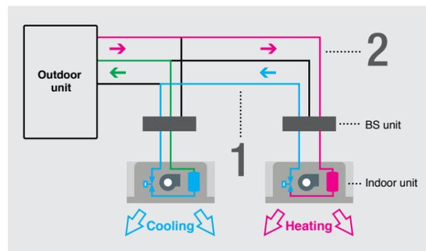
**1** The (cold) waste heat from heating is used for the cooling operation.
