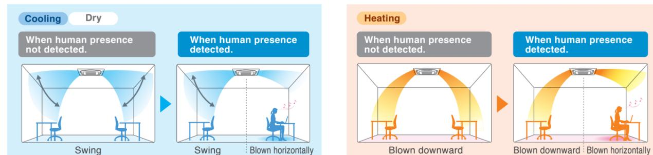
• With the Auto airflow direction mode, flaps are controlled to deliver optimal air distribution for both cooling and heating operations when there are no people.
