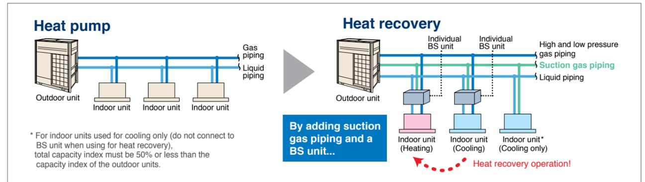
\* For indoor units used for cooling only (do not connect to BS unit when using for heat recovery), total capacity index must be 50% or less than the capacity index of the outdoor units.
