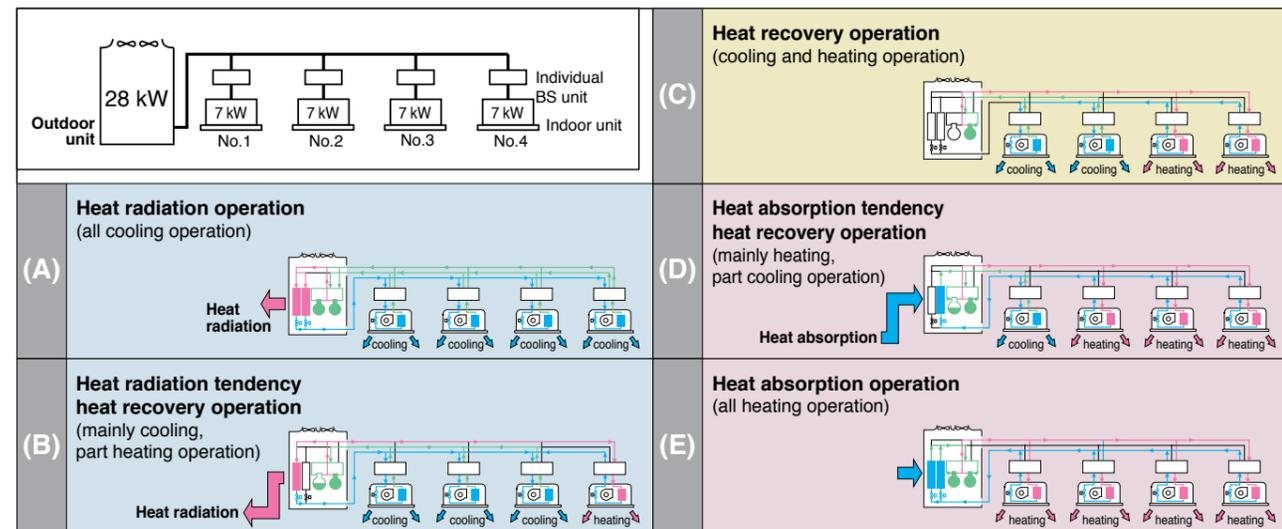
Note: Operation modes (A) and (E) are applicable when the outdoor temperature is 35°C and 7°C respectively; The other modes are applicable under typical outdoor conditions.
