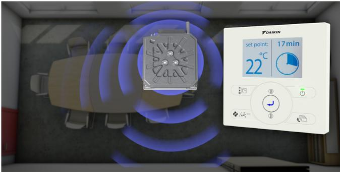
When there is nobody in the room, the presence sensor\* adjusts the set point or switches off the unit, avoiding unnecessary cooling or heating. When motion is detected the temperature is reset to its original setpoint ensuring perfect, energy efficient operation.
